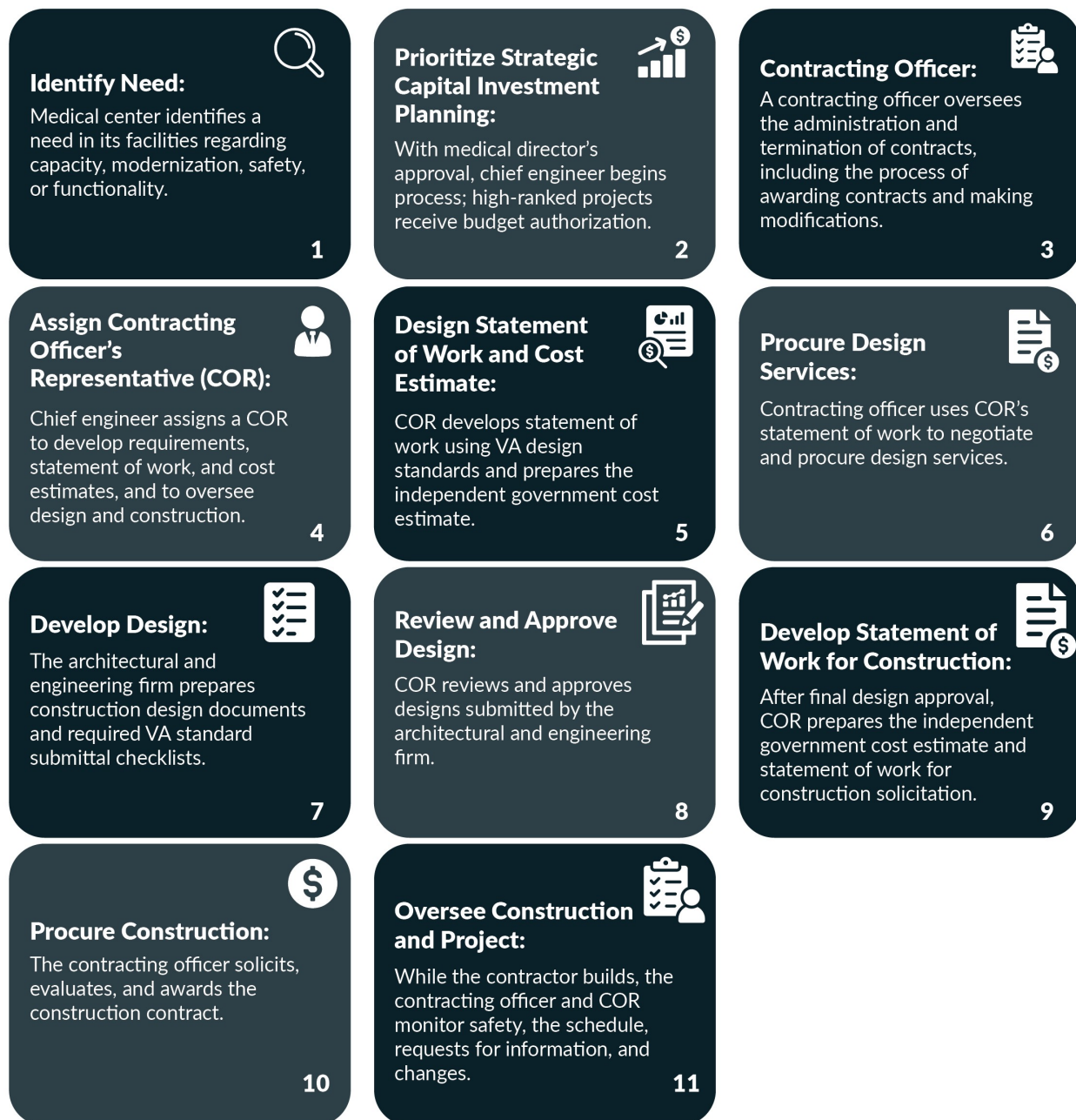
Figure 1. Minor construction and nonrecurring maintenance process.
