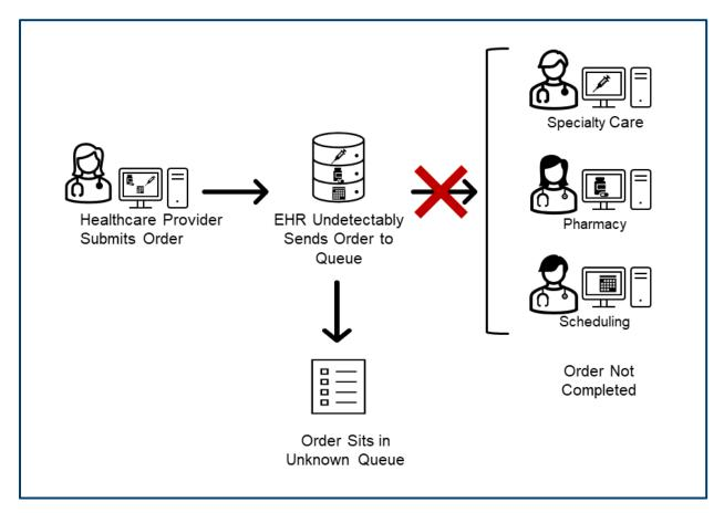
**Figure 4**. Process of the new EHR routing an order to the "unknown queue." Source: OIG analysis.
