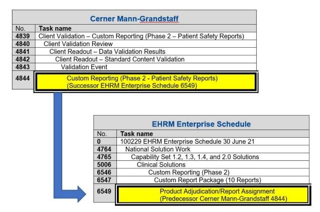
**Figure 1.** Illustration showing how two schedules are linked together through dependencies. Related activities are referred to as predecessors and successors. A predecessor activity must start or finish before its successor.
