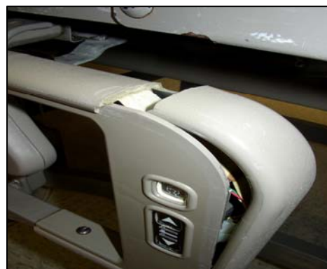
Damaged bed rail with exposed wires
